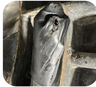
Cable ends were damaged during handling and transit, causing a tear on the end caps.
