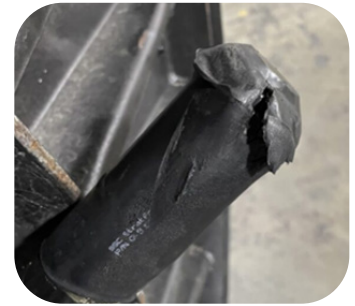
Cable ends were damaged during handling and transit, causing a tear on the end caps.
