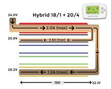
Hybrid Thermostat Cable is designed with an 18 AWG power supply conductor and all remaining conductors at 20 AWG. The smaller gauge conductors use less copper, creating a more cost-effective solution that is lighter and easier to haul.
