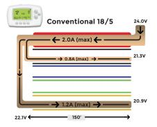
Traditional Thermostat Cable is designed with 18 AWG conductors. Requiring more copper, it is less cost effective and weighs more, making transport more challenging.
