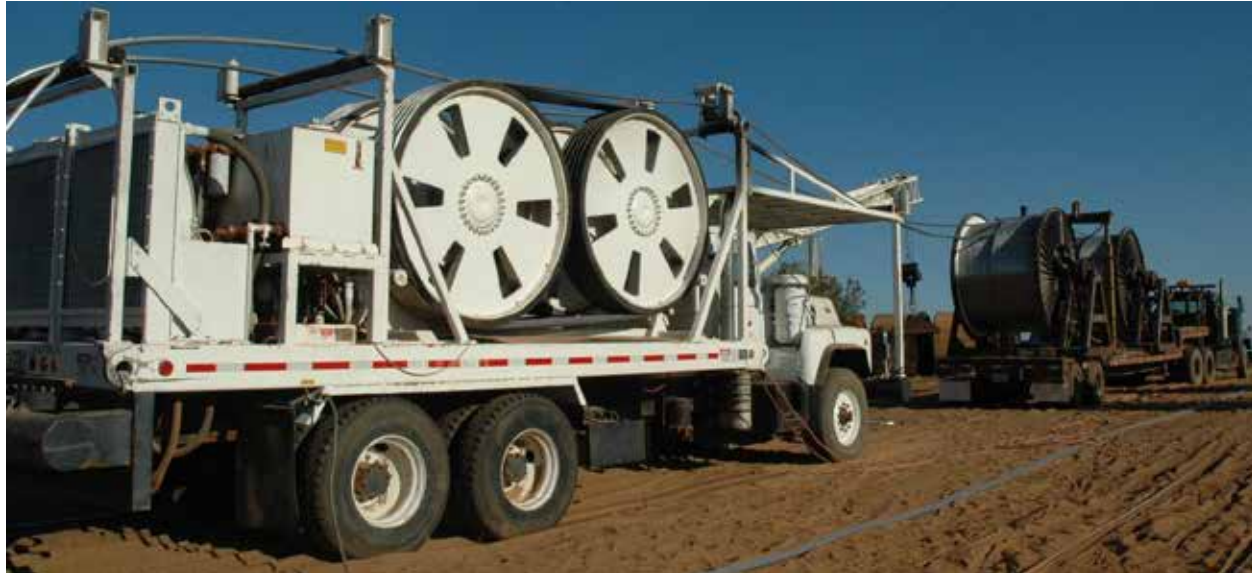
Figure 6. Dual drum bullwheel, courtesy of Oncor.
